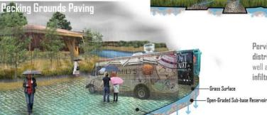
Pervious paving reduces and distributes storm-water volume, as well as encouraging groundwater infiltration.
