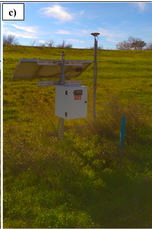
Figure 1. a) Location of in situ GPS stations (approximate coordinates: 38^{\circ}01'56.81'' N, 121^{\circ}45'49.09'' W); b) Installation of pedestal foundation for GPS station; c) completed autonomous GPS station (8003).
