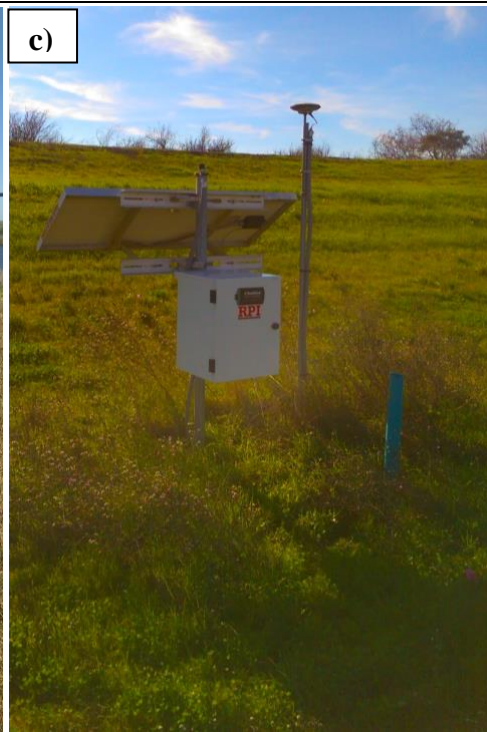
Figure 1. a) Location of in situ GPS stations (approximate coordinates: 38°01'56.81" N, 121°45'49.09" W); b) Installation of pedestal foundation for GPS station; c) completed autonomous GPS station (8003).
