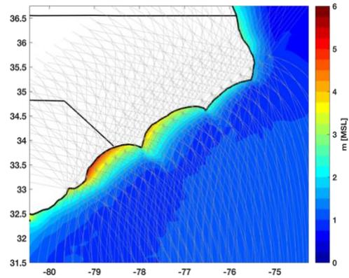
Figure 3. Maximum of maximums across all storms in the new storm population (gray lines), computed on a coarse ADCIRC grid.
