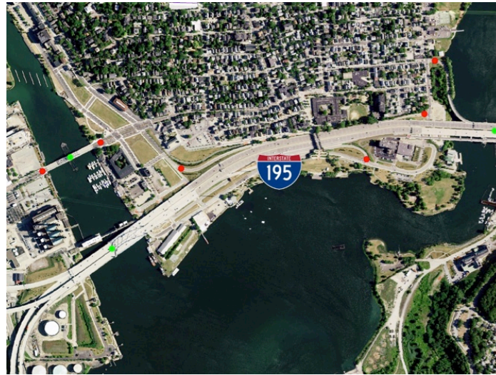
Figure 7.5. Comparison of points located at highway access ramps compared to span centers (green). Before being corrected, span elevation was recorded as the channel bottom (bathymetry). A more logical way to determine whether a span would be compromised would be to ascertain elevation based on the underside of the span (direct impact/shear failure) or at pier locations (scour).
