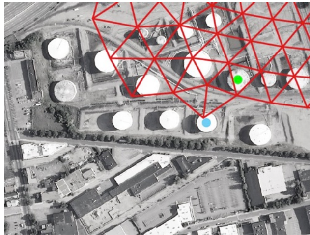
Figure 7.2 Example of a point with three adjacent nodes (green) and point beyond the nearest wet node (blue). The red lines represent wet portions of the unstructured ADCIRC grid. Points tested are both inside and outside of the grid, and constrained by a basin analysis.
