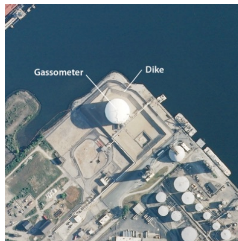
Figure 1.6. Example of micro-topographical condition. The gasometer is protected by an armored concrete dike that is not ‘visible’ to the ocean model. Determining inundation extents without accounting for this dike will lead to misleading results.
