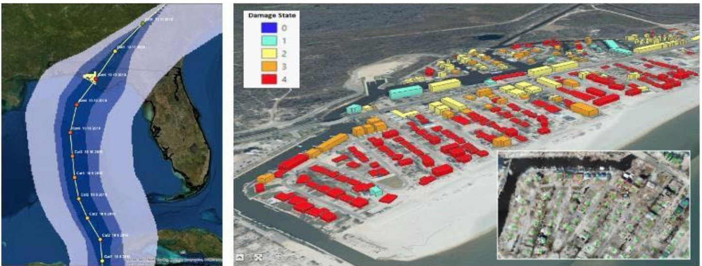
Figure 1: Left: Storm track of Hurricane Michael (2018) making landfall at Mexico Beach, FL. Right: Building damage states from detailed field reconnaissance and aerial imagery (inset) developed during year 6 of this project.
